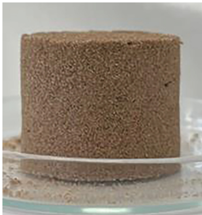
Fig. 5. Example of chitin-sand sample employed for UCS testing.
