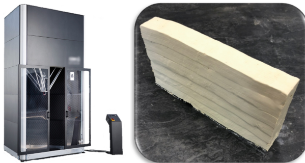
Fig. 3. Printed sample of clay and soy wax with 10 × 30 cm cross section extruder die
