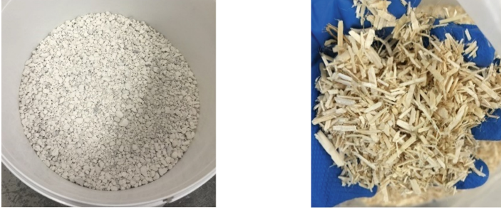
Fig. 1. Quicklime prior to crushing and sieving (left) and hemp shiv.
