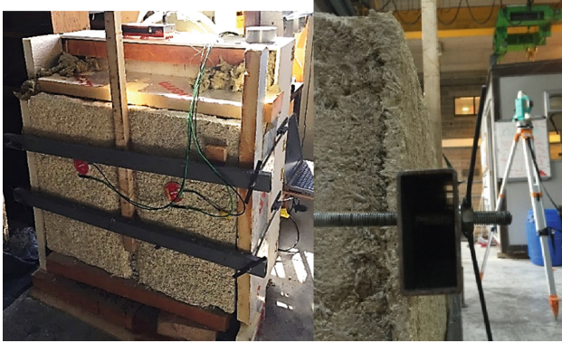
Fig. 2. Hot-box assemblage for thermal conductivity measurement.
