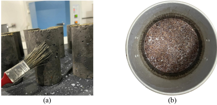
Fig. 1. Silane treatment procedures (a) SSP, and (b) IBA.
