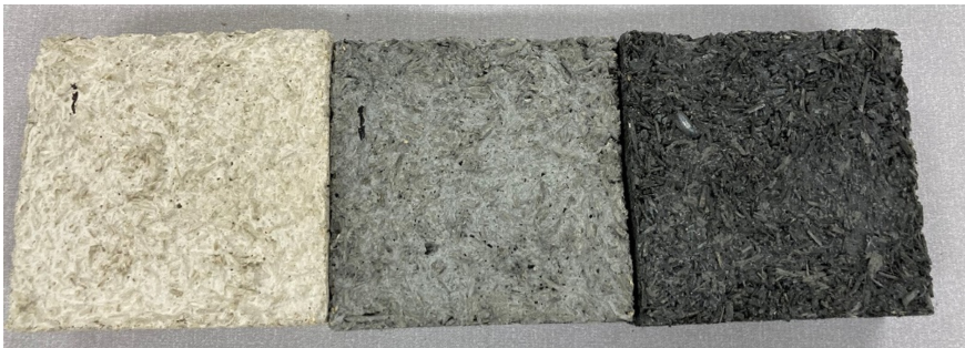
Fig. 5. Left: Hemp-lime, center: Hemp-lime with 20% biochar, right: Hemp-lime with 50% biochar.
