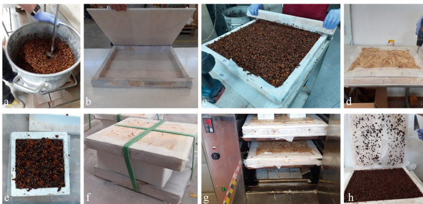
Fig. 5. Production process: a) mechanical mixing; b) wooden mould; c) levelling; d) closure of the wooden mould; e) silicone mould; f) closure of the silicone mould; g) drying at T = 60\text{ }^\circ\text{C} ; h) demoulding.
