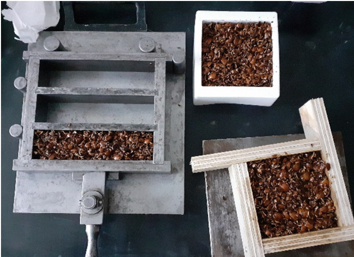
Fig. 3. The considered moulds to produce the samples: metal, wooden and silicone.
