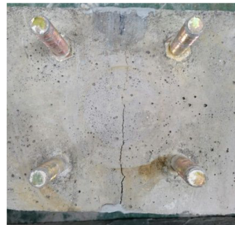
Fig. 7. The formed microcrack.
