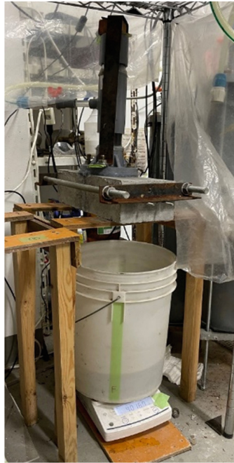
Fig. 8. Water leakage test in progress
