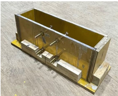
Fig. 4. The specimens of water leakage tests
