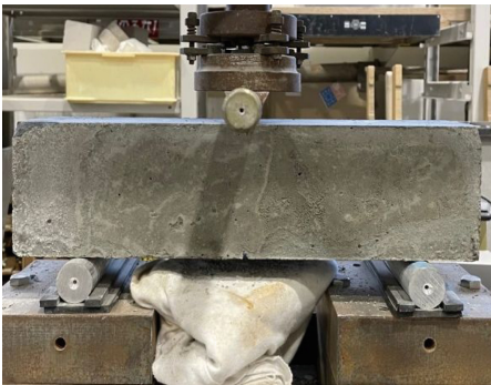
Fig. 6. The state of forming cracks.
