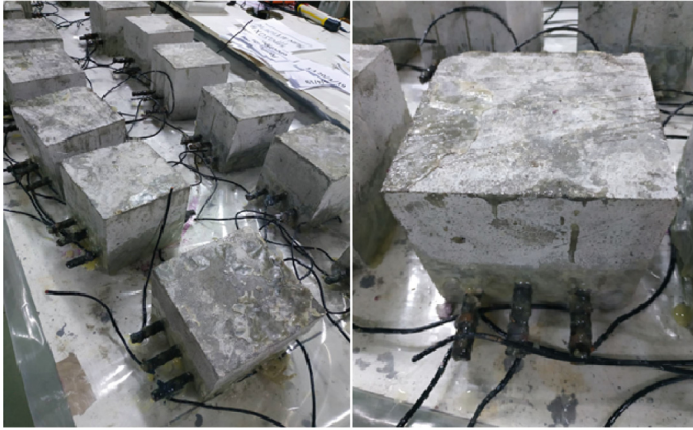
Fig. 1. Reinforced concrete specimens before immersion in NaCl- solution in the laboratory environment.
