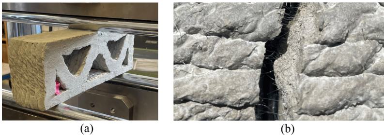
Fig. 3. Test setup of the 3 point bending test (a), and fracture surface of a 3D printed test specimen ( 300 \times 120 \times 100 mm) made of glass fiber reinforced concrete (b).
