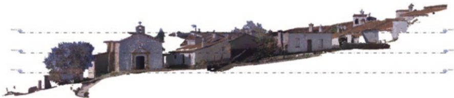
Fig. 2 Longitudinal section in 3D point cloud in the central area of the village. (Source: Own elaboration)
