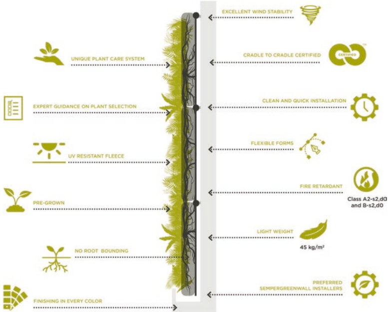
Fig. 6 Characteristics of the green walls. (Image source: Sempergreenwall, 2021)
