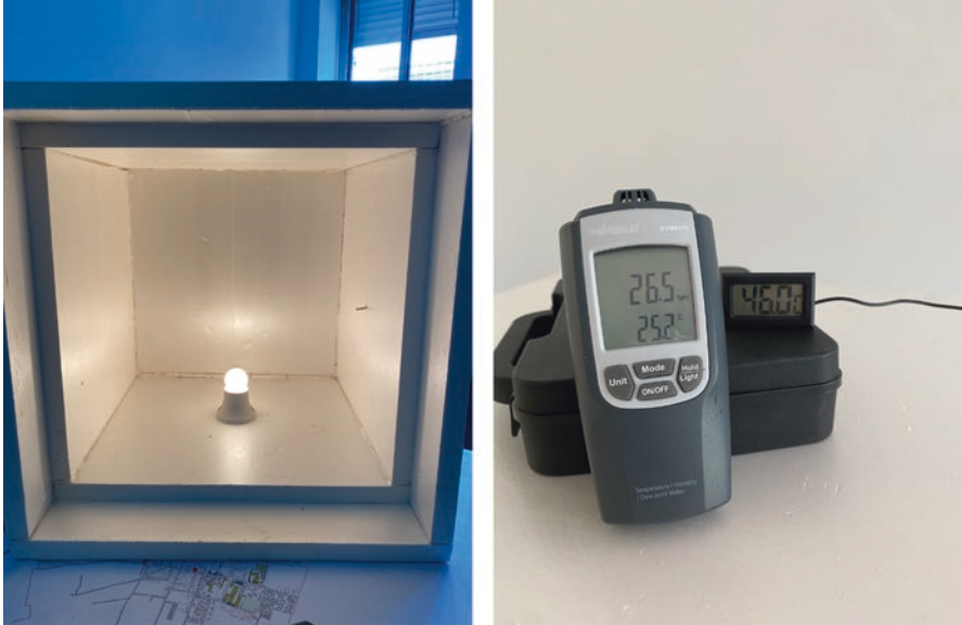
Fig. 2 Left: View of the test box with the heating system on. Right: Thermometer used for the test
