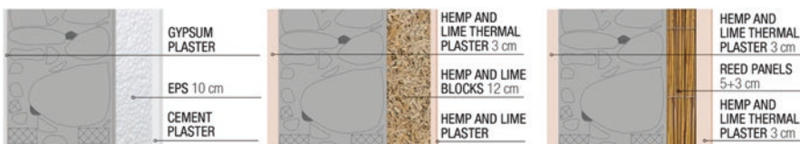
Fig. 3 Wall section and thicknesses of three compared scenarios ( U \simeq 0.34 \text{ W/m}^2\text{K} )
