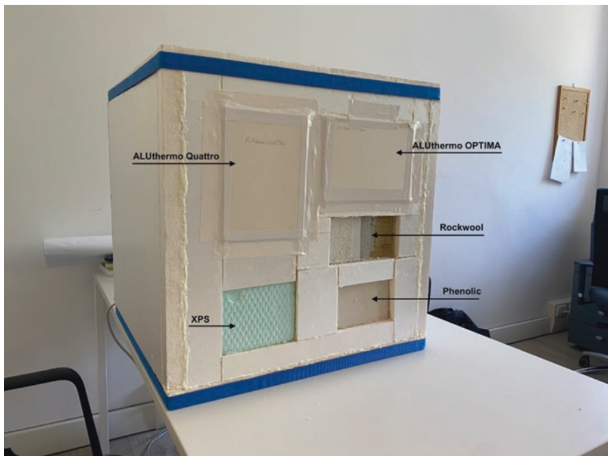
Fig. 3 View of the test box with the side frame holding five different material samples. The top and bottom blue stripes were used to tightly hold in place the front side of the box
