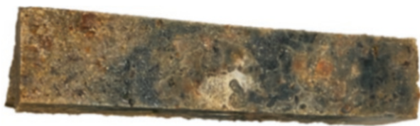
Fig. 2 Decontaminated CCA-treated wood-based geopolymer cement composite
