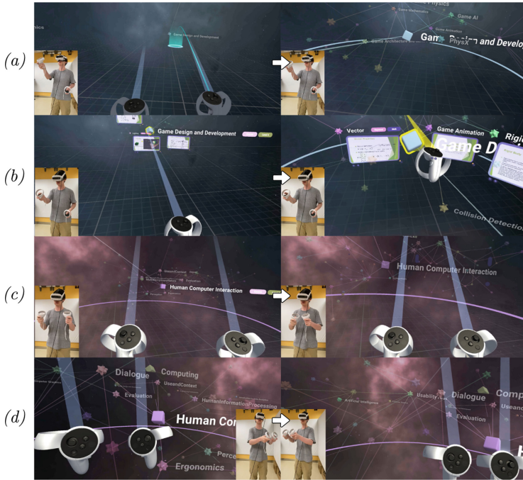
Fig. 5. K-Cube VR can be navigated by (a) spatial teleportation, (b) node teleportation, (c) scaling and (d) translation.
