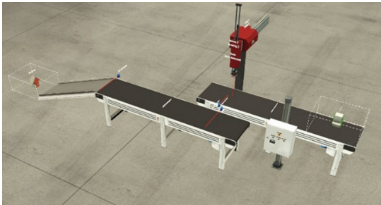
Fig. 3. Creating a robotic workplace in the Factory I/O simulation software.
