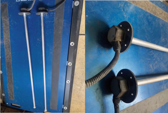
Fig. 2. Fuel level measurement sensor.
