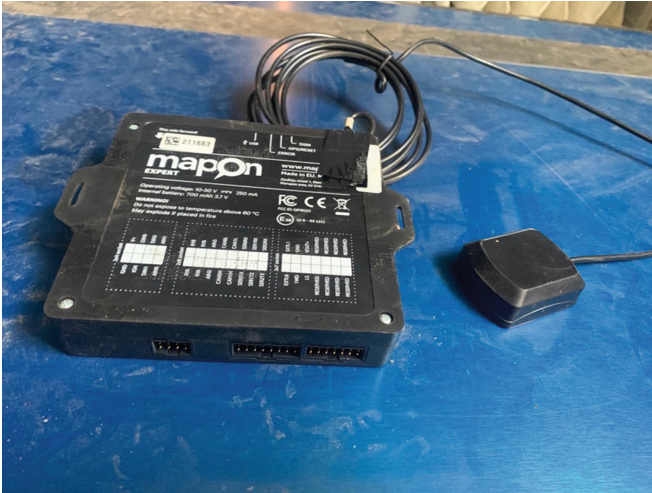
Fig. 1. GPS device - which is installed in the truck.
