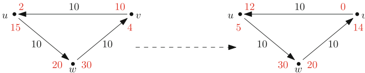
Fig. 2. The graph on the left depicts three nodes u, v, w connected in a cycle. The red numbers by each link represent the capacity of a node in a certain link. u can increase their capacity by 10 on the (u, v) link by first sending the excess capacity of 10 to w along the (u, w) link. Then w sends the excess capacity of 10 to v along (w, v) . Finally, v sends capacity of 10 back to u along (v, u) . The graph on the right depicts the updated capacities of each node on each link after cyclic redistribution. (Color figure online)
