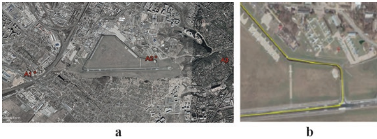
Fig. 11.3 Location of additional receivers A1-A3 (a) and track (yellow) correspondence to runway and taxiways geometry (A2) (b)
