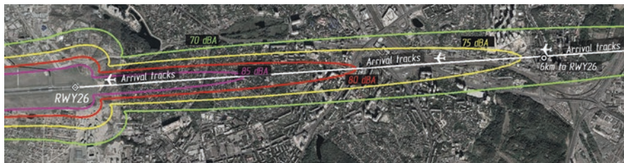
Fig. 11.4 Track dispersion (white lines) during descent and arrival procedures, typical for city airport; 70–85 dBA are L Amax noise levels
