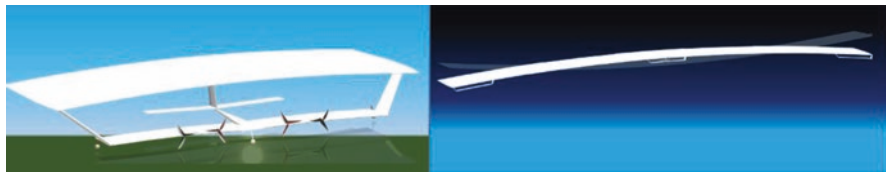
Fig. 16.1 1 (Left) 32 m \times 4 m, 4-propeller FLT with partially deployed sheet above. (Right) 353 m \times 32 m FL
