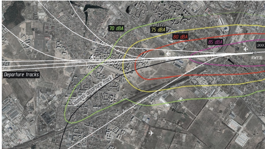
Fig. 11.5 Dispersion of takeoff tracks for the same flight and its impact on the form of noise contours L_{Amax} = 70 \dots 85 dBA; A320, October 2021
