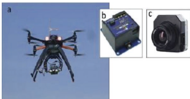
Fig. 26.1 (a) UAV platform designed for imaging; (b) multispectral; and (c) thermal camera systems
