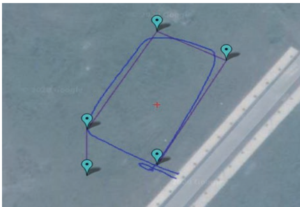
Fig. 25.1 Blue line – real trajectory; purple line – requested trajectory
