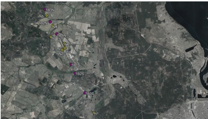
Fig. 21.1 Location of AN measurement points in the vicinity of Kyiv/Gostomel Airport (yellow points – for departures; pink points – for arrivals)
