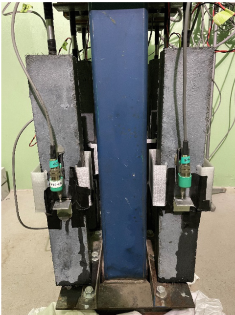
Fig. 1. Test set-up of specimens under constant loading
