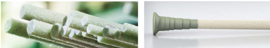
Fig. 1. FRP materials accepted by CSA S807 [1] (Courtesy of PohlCon GmbH, Germany).
