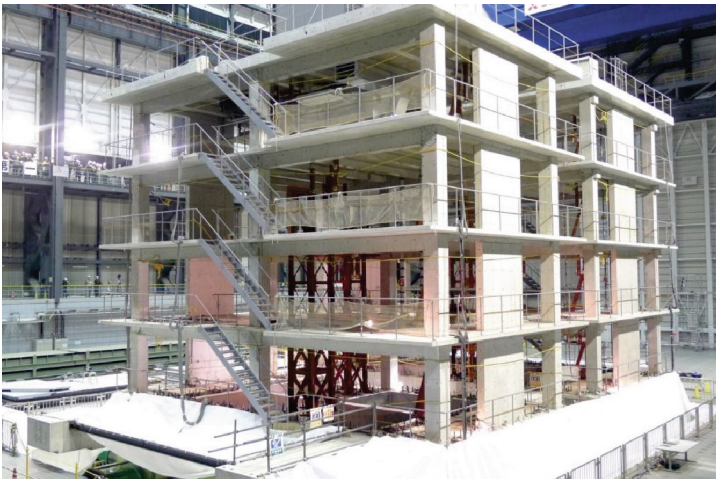
Fig. 1. Four-story RC structure tested at E-Defense shake table 2010. [4]
