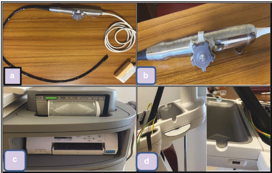
Fig. 2 Photo of a transducer. (a) Transducer bad, (b) handle, control wheels, and brake; (c) printer unit; (d) recording unit
