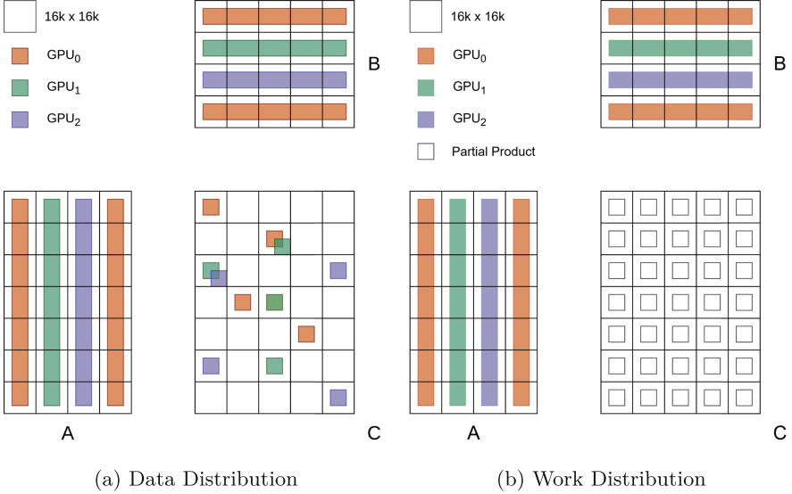
Fig. 1. (a) represents the data distribution. For each GPU, only 1 column of tiles from A and 1 row of tiles from B are considered at a time. For matrix C, each GPU gets p partial product tiles (reusable), for storing the partial GEMM computations. (b) represents the work distribution on the GPUs. It is quite similar to the data distribution, where each GPU calculate the partial result for all the elements in matrix C.
