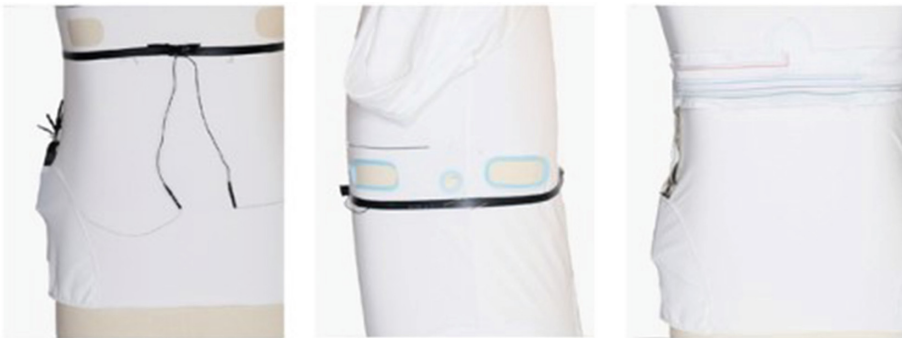
Fig. 5. Focus on wearable add-on Smart T-Shirt. Focus on arrangement of conductive yarns by color and type of sensor connection; study of electronics components to operation and monitoring of vital parameters (Sbordone et al., Smart&Safe Project 2020).
