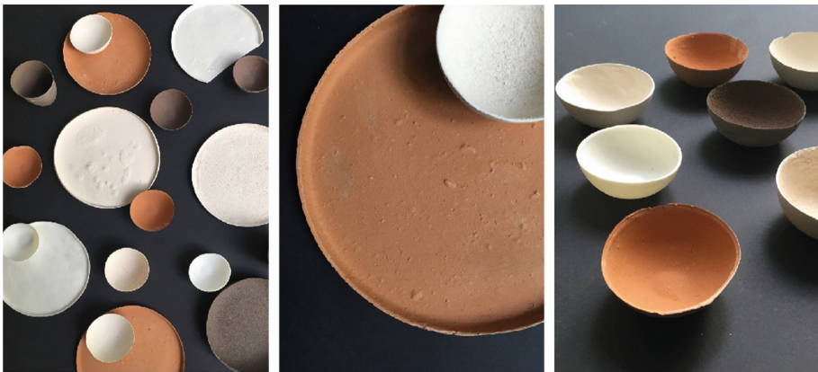
Fig. 8. Objects made of clay+algae were created to understand the expressive sensory characteristics of the new material and its behaviour during the forming processes.
