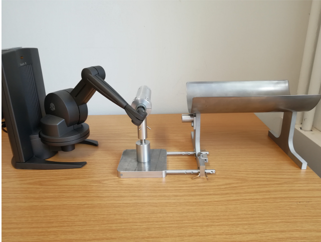
Fig. 4. System in the configuration for the ulnar and radial deviation game-mode
