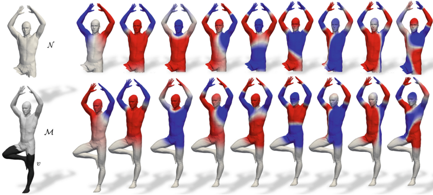
Fig. 1. Top: First eigenvectors of the LBO of the partial shape \mathcal{N} . Bottom: First eigenvectors of the Hamiltonian of the full shape \mathcal{M} . The Hamiltonian is defined with a step potential v (in black) corresponding to the effective support of \mathcal{N} . With the potential v , the eigenfunctions of the LBO and the Hamiltonian are similar up to a sign.
