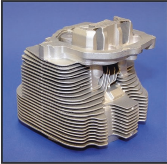
Fig. 14.9 Air-cooled cylinder head poured from Al-Ce binary alloy
