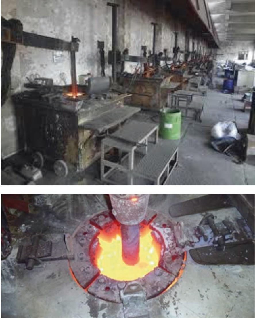
Fig. 9.12 Neodymium cell. (Cell was operated by Great Western Resources which has a W cathode center electrode [29])
