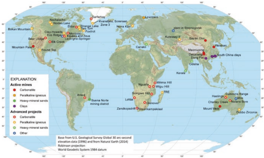
Fig. 2.6 Global distribution of active REE deposits and advanced projects by deposit type. (Compiled for 2017 [20])
