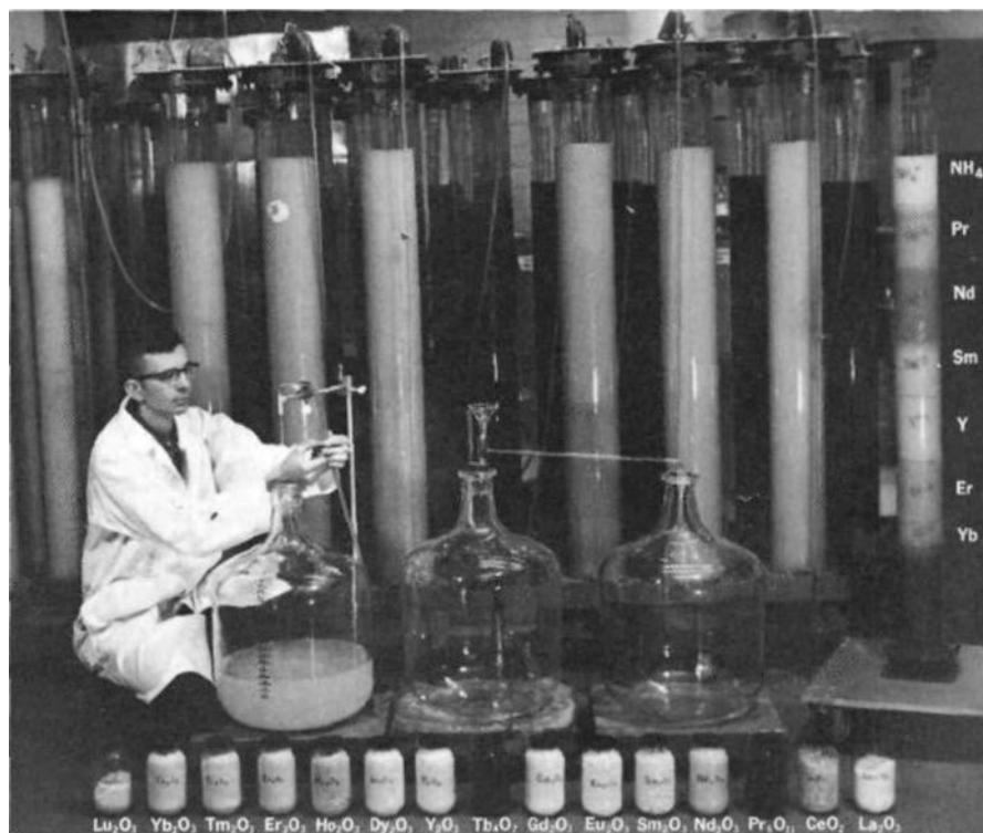
Fig. 7.1 Ion exchange columns used to separate the rare earths from one another. Individual rare earths are collected in the large carboys as they are removed from the columns. The jars in front of the chemist contain the oxides of the individual rare earth elements [3]
