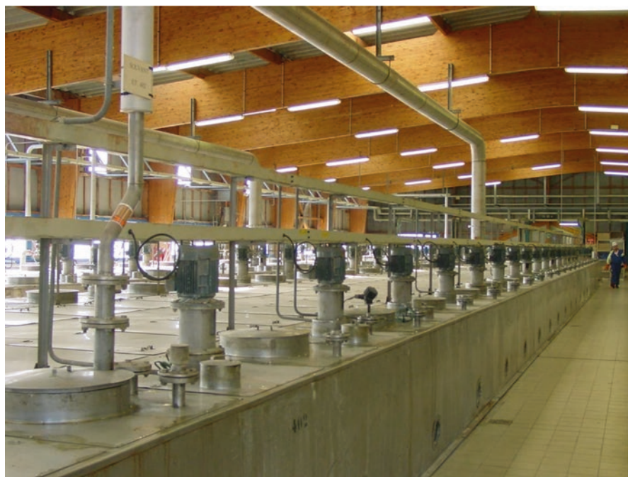
Fig. 6.12 Rare earth solvent extraction battery in Solvay La Rochelle plant in France. (Photo from SoS RARE - Copyright Solvay)
