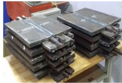
(c) Joint after welding
