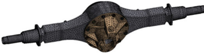
Fig. 2 Rear axle housing’s meshing model
