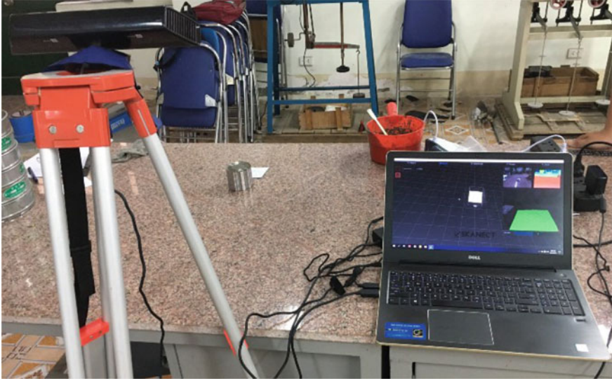
Fig. 2 Utilization of the depth sensor during the slump and slump-flow test
