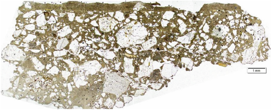
Fig. 3. The coloured intonaco layer is composed of fine-grained binder with occasional binder related particles and an aggregate - predominantly quartz and gneiss. The lime wash does not contain filler and appears as one about 0.2–0.4 mm thick single layer. Sample OSL 4, PPL.
