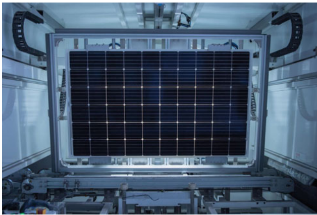
Fig. 29 Flash test of assembled PV panel (Findlay 2022)
