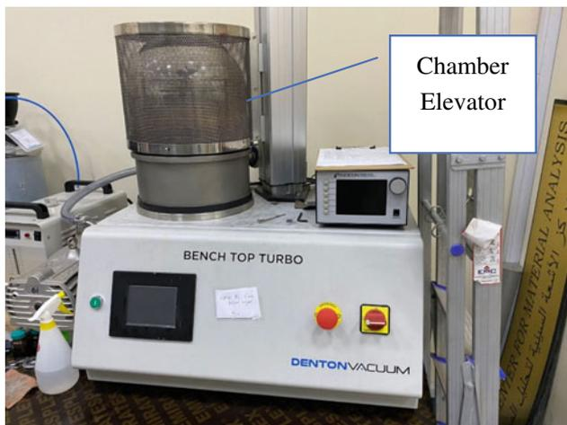
**Fig. 24** Thermal evaporator
