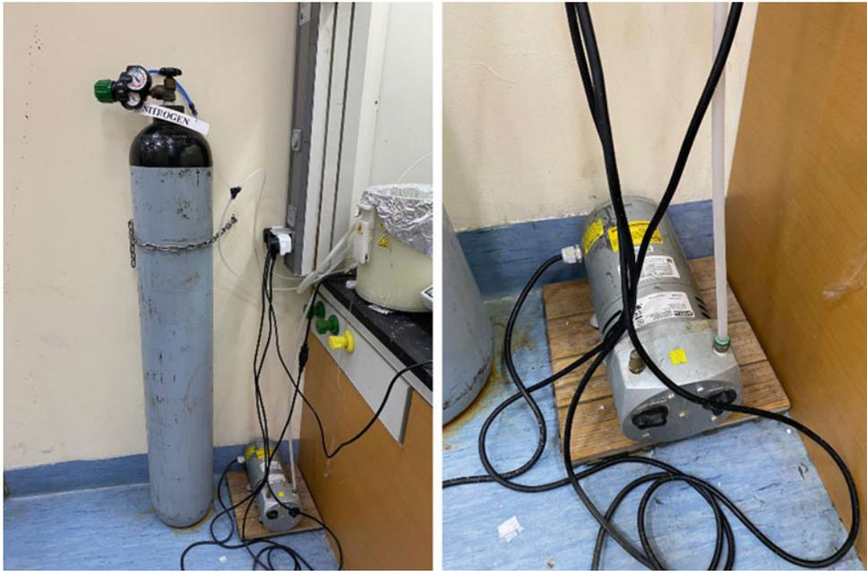
**Fig. 9** Spin coater vacuum system-nitrogen tank—compressor
