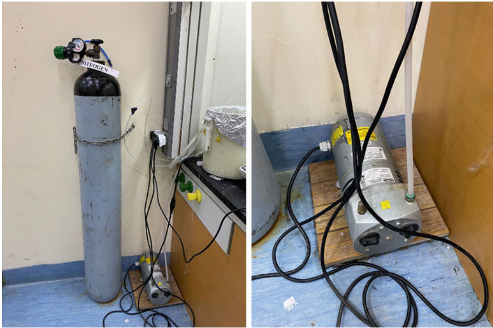
Fig. 9 Spin coater vacuum system-nitrogen tank—compressor
