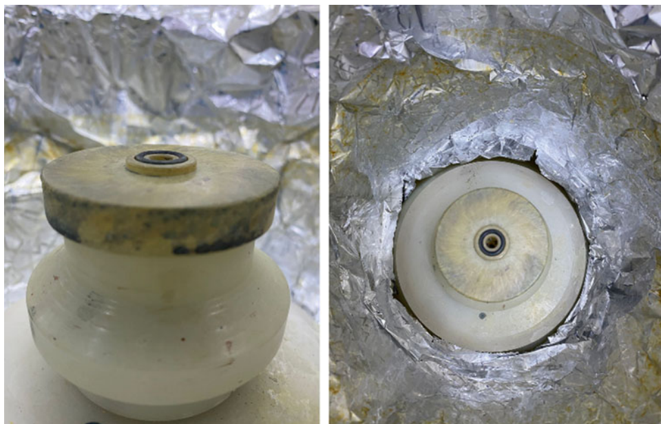
Fig. 8 Vacuum-assisted substrate holder—side and top view
