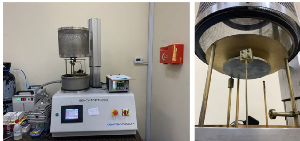
Fig. 25 Thermal evaporator glass chamber with protective mesh around it a open and b closeup
