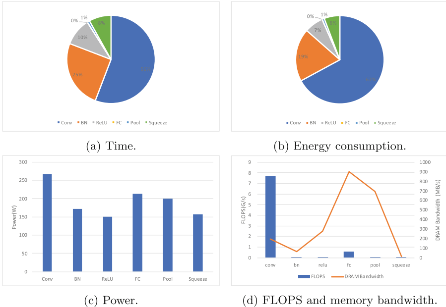
Fig. 4. Layer analysis of ResNet50.
