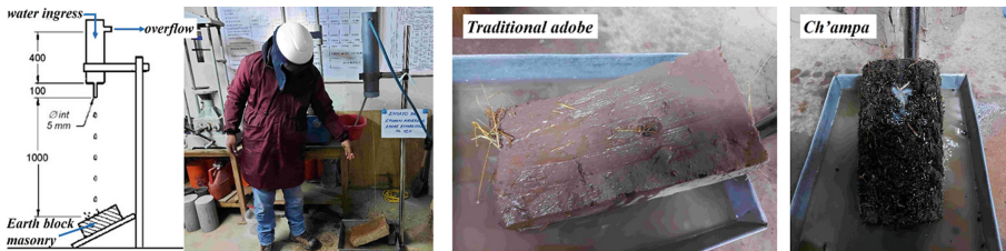
Fig. 5. Swinburne accelerated erosion (SAET) for traditional adobe and Ch'ampa blocks.
