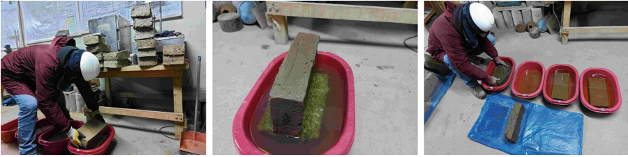
Fig. 3. Immersion of traditional adobe and Ch'ampa blocks.
