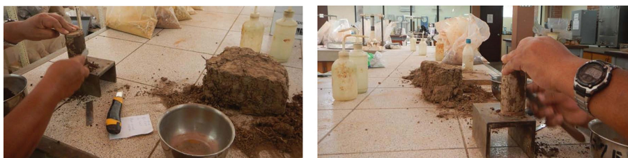
Fig. 2. Molding of samples P-1 and P-2 for permeability test.
