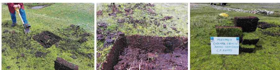
Fig. 1. Extraction of the Ch'ampa samples using the same artisanal criteria of the study area.
