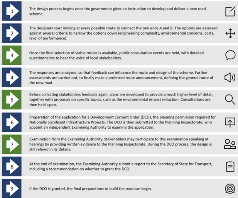
Fig. 3 Approval process in the UK. Non-market stakeholders are directly involved in the green steps
