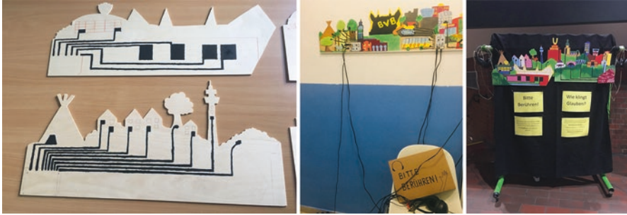
Fig. 3.1 The city of sound was crafted from wood. Equipped with programmable micro-boards, it could produce sound upon touch of designated spots which were marked with conductive paint
