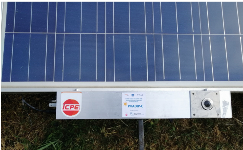
Fig. 4. The Dr. Solar box fixed to the solar panel
