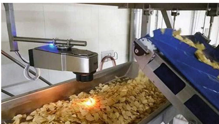
Plate 12.1 In-line NIR instrument based on diode array technology for continuous measurement of seasoning addition, moisture and fat content in snack foods; Photograph courtesy; Perkin Elmer. ( https://www.perkinelmer.com/uk/libraries/app_measuring_seasoning_addition_in_snackfoods_da7440 )
