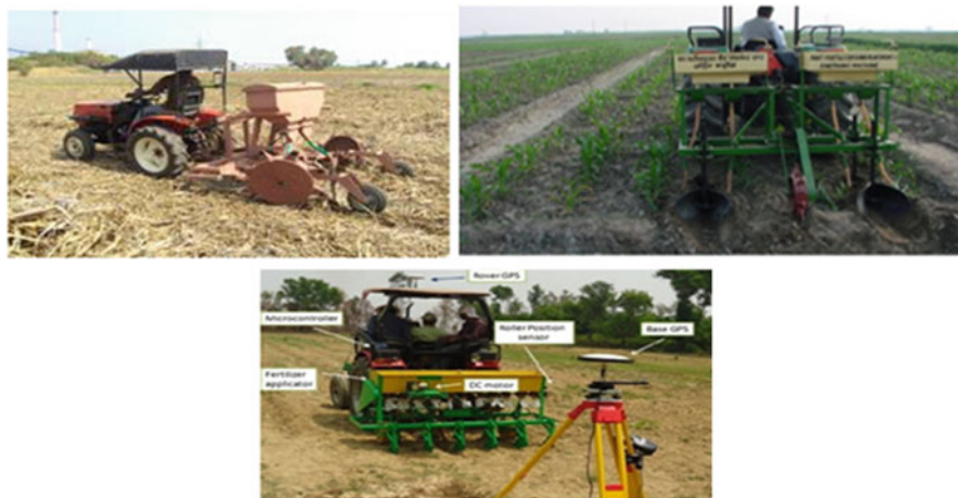
Fig. 5.6 Mechanized fertilizer application equipment (a) Tractor-operated fertilizer dibbler (b) Fertilizer band placement cum earthing up the machine (c) GPS based variable rate granular fertilizer applicator. (Source-AICRP – FIM)
