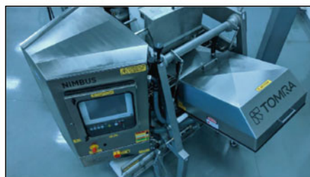
(b) TOMRA Nimbus 640 with double Laser in DETOX™ Configuration
