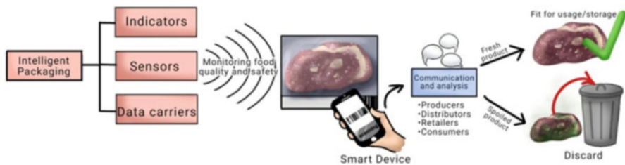
Fig. 14.1 Illustration of the application of IP systems for monitoring food quality and safety
