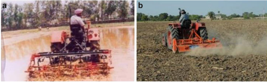
Fig. 5.2 Mechanized seedbed preparation equipment (a) Tractor mounted pulverizing roller attachment to tiller (b) Tractor mounted rotary tiller. (Source-AICRP – FIM)
