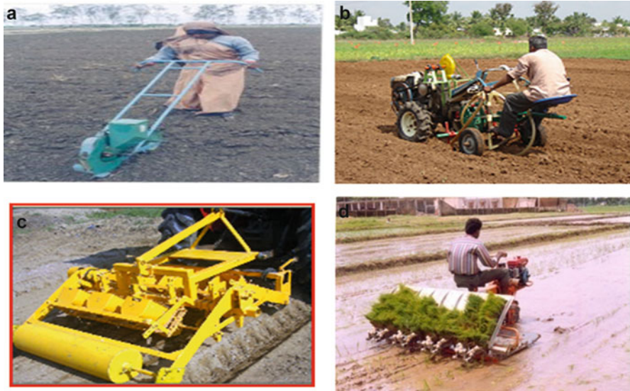
Fig. 5.5 Mechanized seedling application equipment (a) Rotary dibbler (b) Power tiller mounted air assisted seed drill (c) Tractor Operated Small Seed Planter (d) Self-propelled rice transplanter. (Source-AICRP – FIM)
