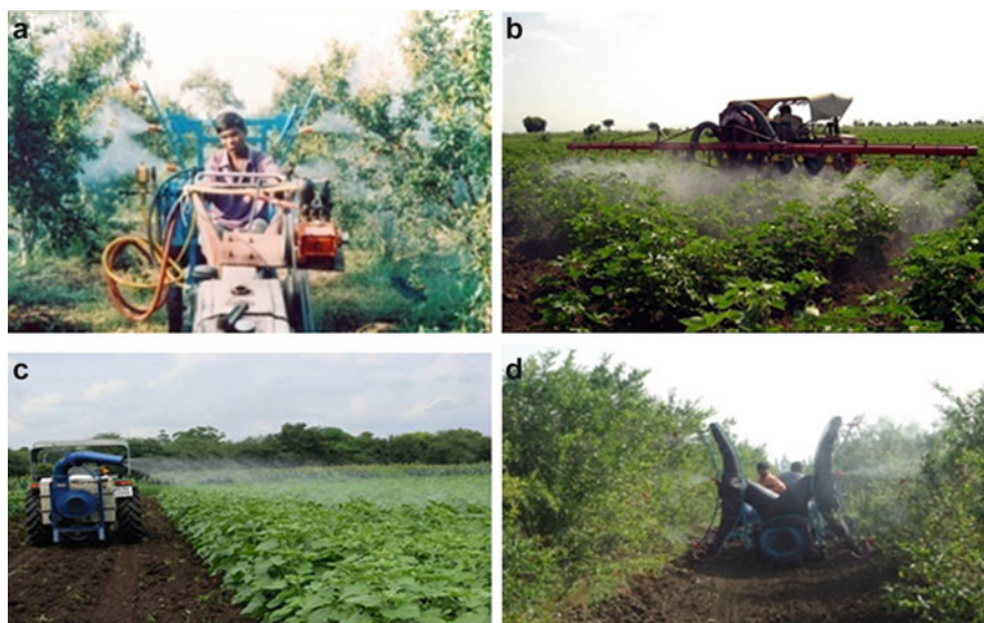
Fig. 5.7 Sprayer application equipment (a) Multi orchard sprayer (b) Tractor mounted boom sprayer (c) Tractor operated aero blast sprayer (d) Ultrasonic sensor based spraying system. (Source-AICRP – FIM)
