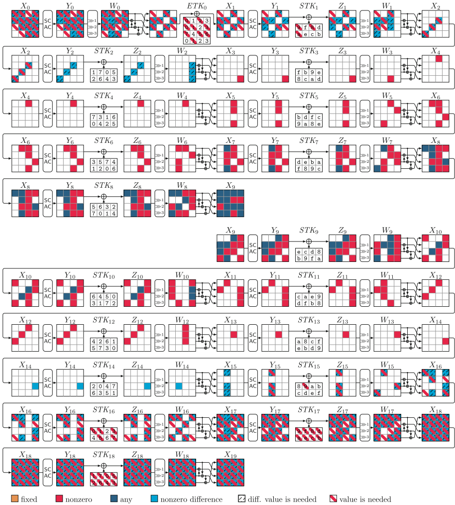
Fig. 4. ID attack on 19 rounds of SKINNY [n-2n] , |k_B \cup k_F| = 26 \cdot c , c_B = 6 \cdot c , c_F = 15 \cdot c , \Delta_B = 7 \cdot c , \Delta_F = 16 \cdot c
