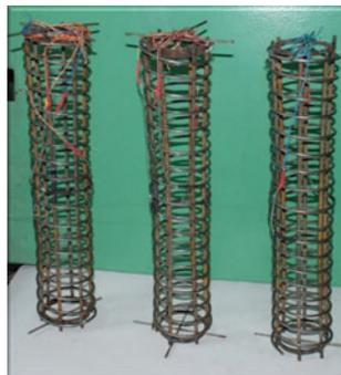
**Fig. 2** Frames with spiral reinforcement for installation in square-section tube-concrete structures
