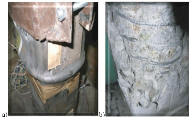
**Fig. 14** Samples view of the SA-80 series after destruction: **a** - the formation of a fold on the shell side surface; **b** - spiral rupture
