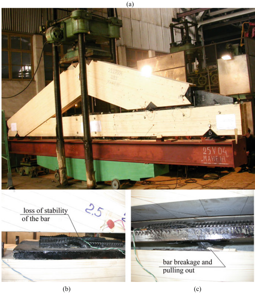
Fig. 4 Control tests of the experimental sample of the TSVZ “Manezh” truss: (a) general view; (b) loss of stability of the compressed rod at failure; (c) rupture and pulling out of the stretched bar
