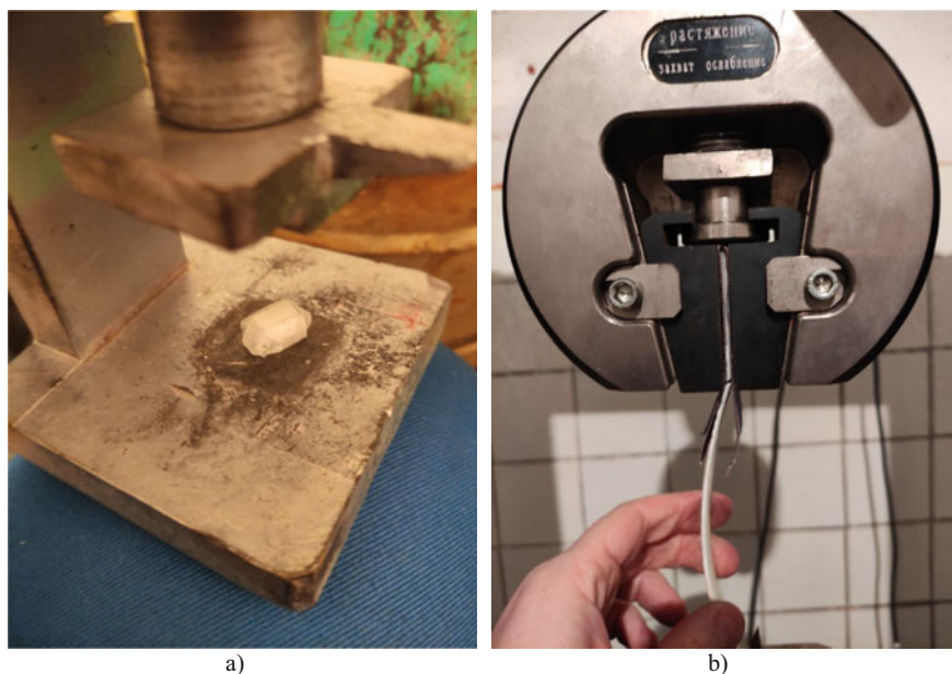
Fig. 4 Destruction of polymer composition samples: a for compression; b for stretching
