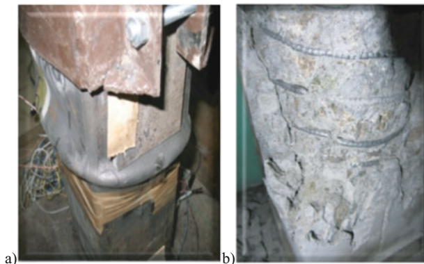
Fig. 14 Samples view of the SA-80 series after destruction: a - the formation of a fold on the shell side surface; b - spiral rupture
