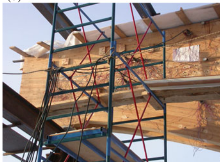
Fig. 8 Control tests of a block of two lenticular trusses with a span of 48 m: (a) general view in the process of loading; (b) load cells in the supporting zone; (c) pushing through the bars with subsequent crushing on the support
