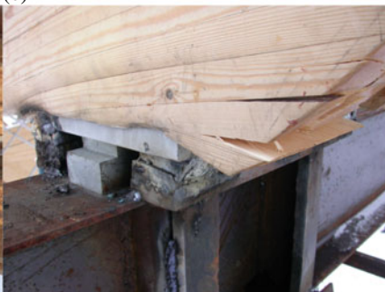
Fig. 8 Control tests of a block of two lenticular trusses with a span of 48 m: (a) general view in the process of loading; (b) load cells in the supporting zone; (c) pushing through the bars with subsequent crushing on the support
