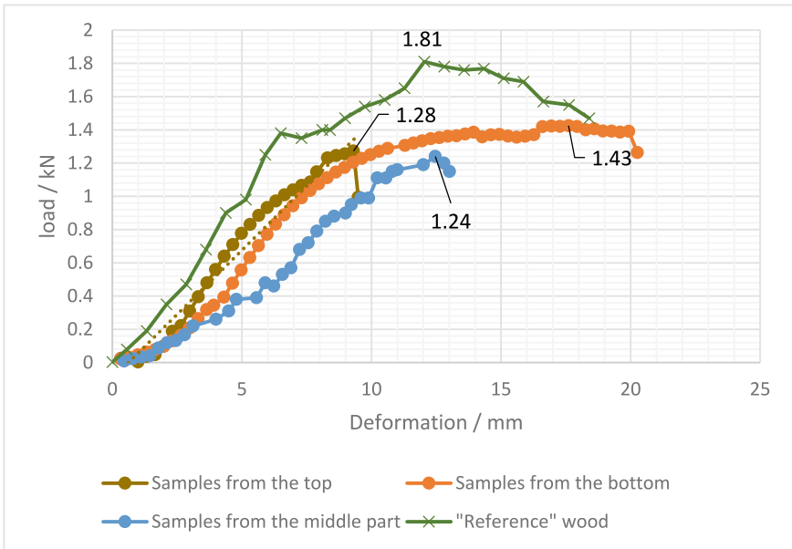
Fig. 7 Results of testing specimens for static bending. Namtsy-1 Khomustakh
