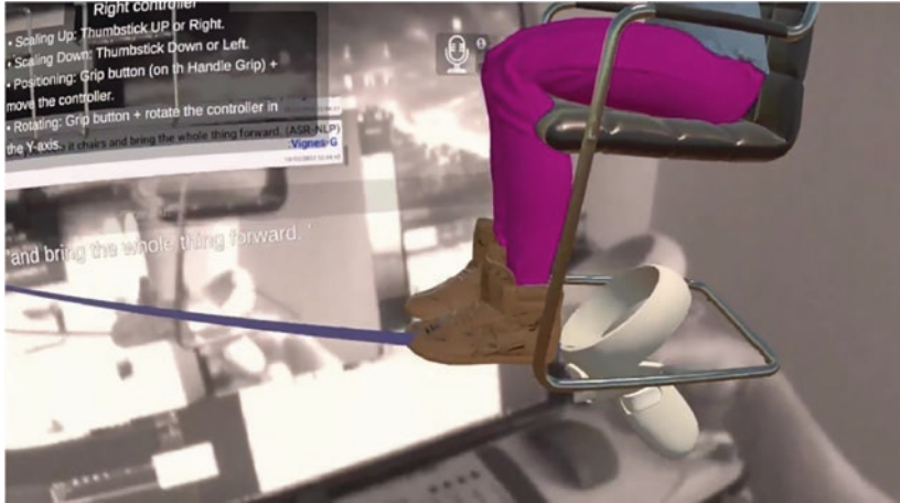
Fig. 5 In MR mode, the user's avatar and chairs are scaled, positioned, and rotated in the Y-axis next to the computer screen. Positioning and rotation are done using the hand-held controller's position and rotation. In this case, the right-hand controller is visible in the background. It is possible to observe that the hand is bending to rotate the controller for avatar and chair rotation in the Y-axis. This is a render buffer capture using SideQuest software
