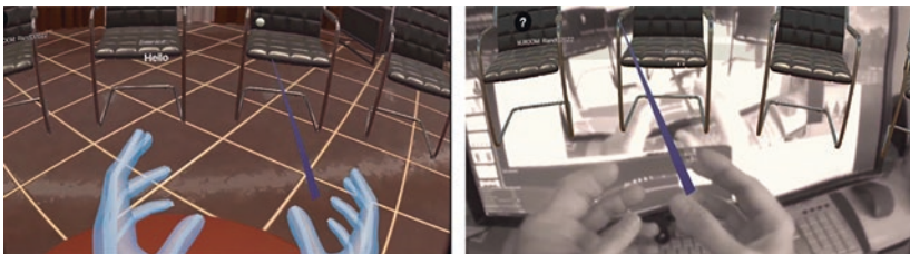
Fig. 4 Left: Hand tracking in VR mode with the Oculus Quest 2. Here, the right hand has the pointer, which means it is controlling, active, or dominant. Right: Hand tracking in MR mode with the Oculus Quest 2. Here, the camera feed of the actual hands are visible, and the right hand has the pointer, which means it is controlling, active, or dominant. This is a render buffer capture using SideQuest software
