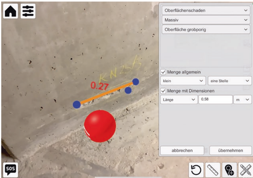
Fig. 2 Damage sphere with measurement tool and input form (screenshot from our prototype)
