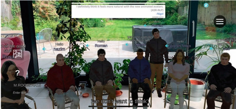
Fig. 1 AR Mono application mode, where the computer-generated imagery (CGI) is augmented onto the actual real-world video stream and rendered in a standard display
