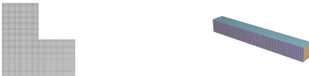
Fig. 2. Meshes used for MFEM diffusion experiments. Left: L-shape mesh with 7 levels of uniform refinement (49,152 elements); Right: Beam mesh with 3 levels of uniform refinement (4,096 elements).
