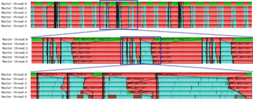
Fig. 5. Tracing from a number of iterations of the optimization. Rank 0 handles the optimization solver (green is time spent in IPOPT) while the other ranks do the function evaluations where cyan is sparse linear algebra operations (to compute the dose), red is time waiting for the optimization solver, and the brown is computing function values from the dose. In the second panel we zoom in and show three evaluations. In the third panel the different stages of the objective function evaluation are clearly distinguishable. (Color figure online)
