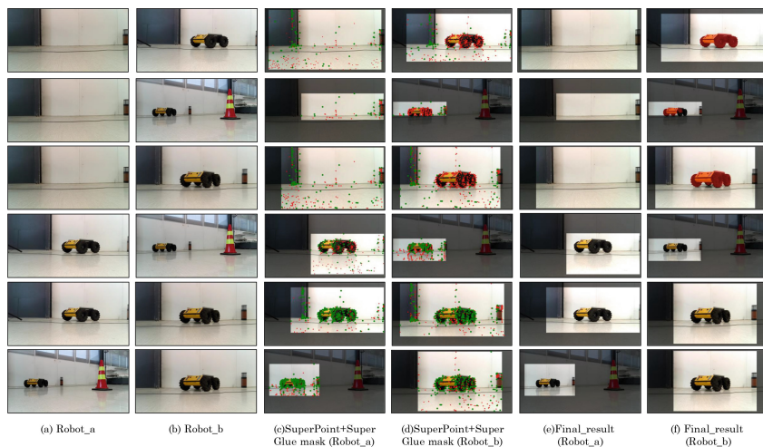
Fig. 5. Comparison of pair images related to the required locations by IOTA smart contract. The first two columns represent images submitted by robots. After feature extraction and clustering, the final results represent different robot pairs.
