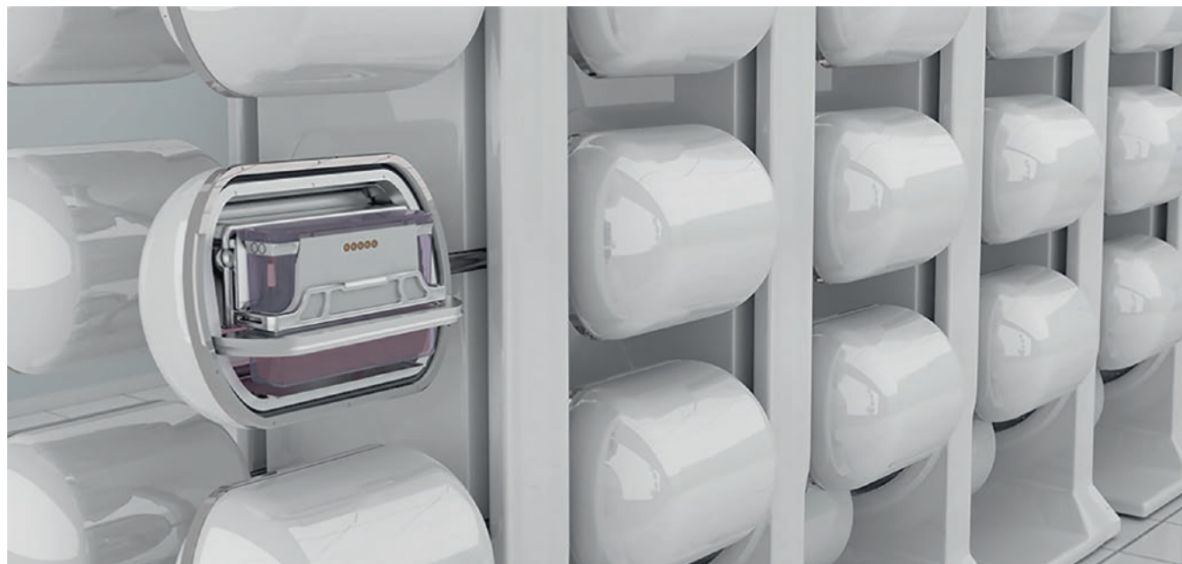
Fig. 14.31 Octane Technology, a fully closed production system for scale-out of autologous or allogeneic tissue- and cell-based products
