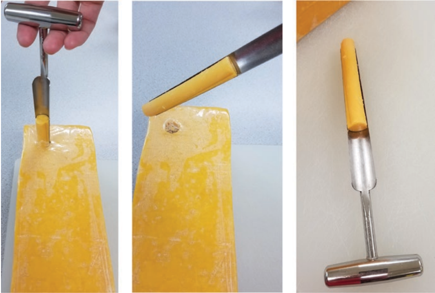
Fig. 9.4 Removing a cheese plug from a 5-lb block of Cheddar with a 127-mm (5-in) trier. (Stephanie Clark images)
