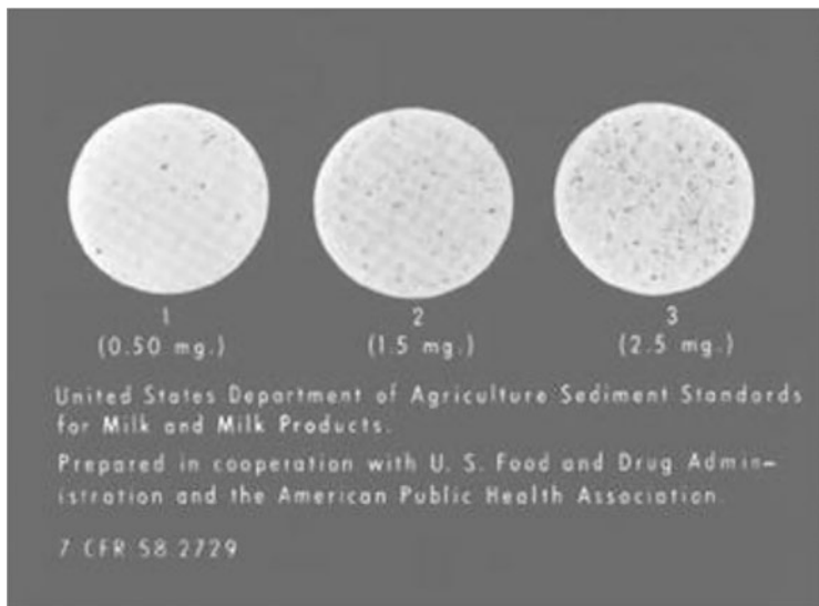
Fig. 5.5 Standard discs that represent known weights of sediment for a given volume of tempered milk sample (one pint)
